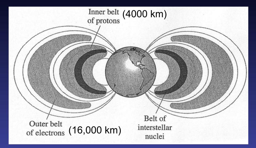
The Van Allen radiation belts arise from charged particles trapped in the magnetic field of Earth.
