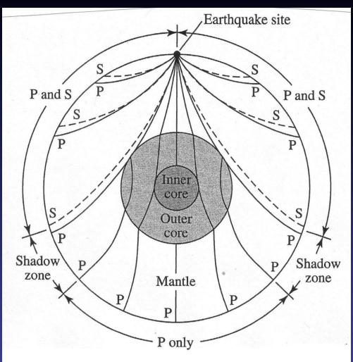
The propagation of S and P waves depends on the density and state of the medium. The state depends on temperature and pressure. Solid inner core, molten outer core, thick mantle.
